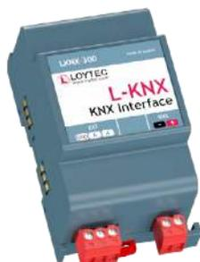
The KNX-Interface LKNX-300 allows the L-INX Automation Servers, the L-ROC Room Controllers, and the L-GATE Universal Gateways to interface to KNX devices connected to a KNX TP1 Bus. The LKNX-300 Interface needs to be connected to the EXT-Port on the L-INX/L-ROC/L-GATE devices.
